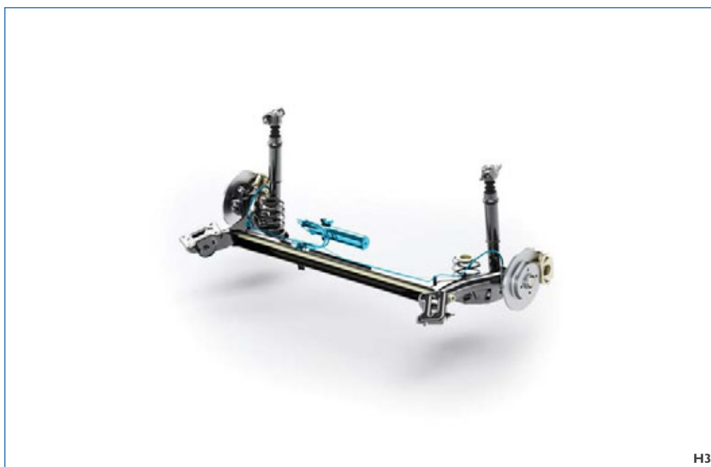
H3 : Close up of rear suspension with the Dynamic Roll Control system
