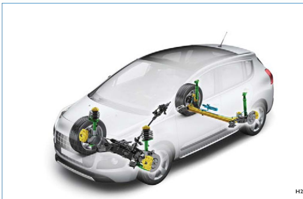
H2 : Chassis and suspension with Dynamic Roll Control system
